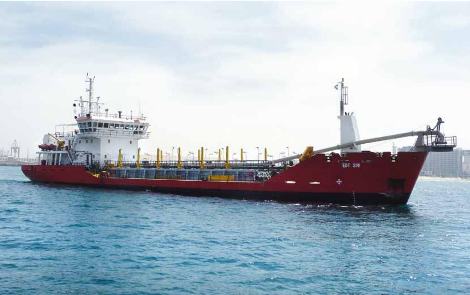
The sand dredger EDT SIMI, built in 1999, measures 70.75 meters in length and can hold 5,000 tons of cargo. It sails under the flag of Cyprus, dredging sand from a depth of 10 to 30 m in bodies of water all over the world. 1,600 m<sup>3</sup> of sediment can be conveyed in less than 2 hours via its suction hose. In the same period, 1,200 m<sup>3</sup> of cargo can be discharged on land.
