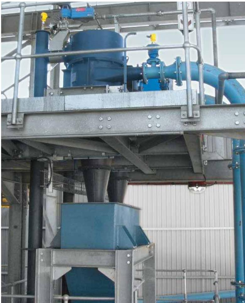
Rock residues are separated from the usable iron ore by centrifugal force in the hydrocyclone.
