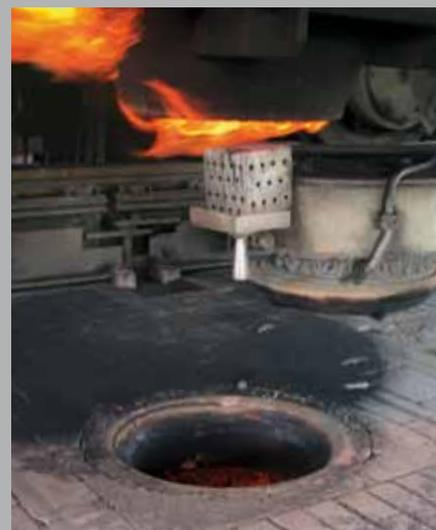
Extreme radar level measurement of red-hot coke: level measurement in the coke oven optimizes the filling process during degassing.
