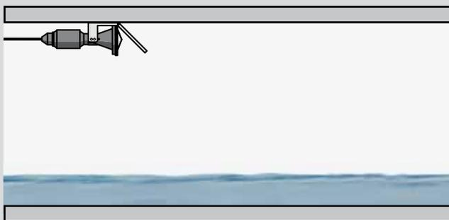
Measuring around the corner with VEGAPULS WL 61: a suitable holder with integrated deflection plate for fast, space-saving installation.
