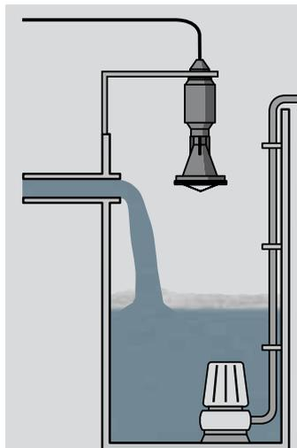
The VEGAPULS WL 61 is perfect for measurement in wastewater environments: simple mounting, encapsulated construction and high protection rating.
