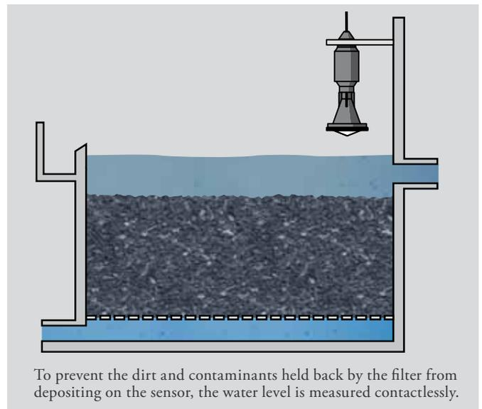
VEGAPULS WL 61 radar sensors are used to monitor the water levels in the 40 carbon filter pools of Waternet. Mounted directly on the basin wall, they detect the level continuously without touching the medium – fouling of the sensors is impossible. Also, any contaminants on the surface of the water or foam generation during the flushing process don't affect the measurement.
